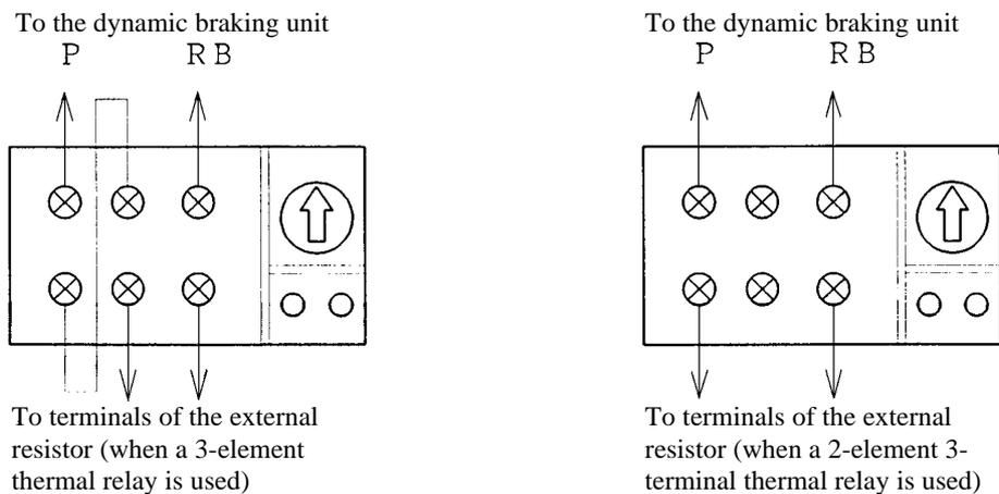
Figure 4.2 Connection of a Thermal Relay
