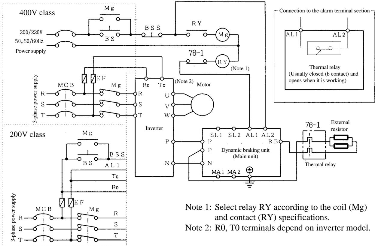
Figure 4.1 External connection example
