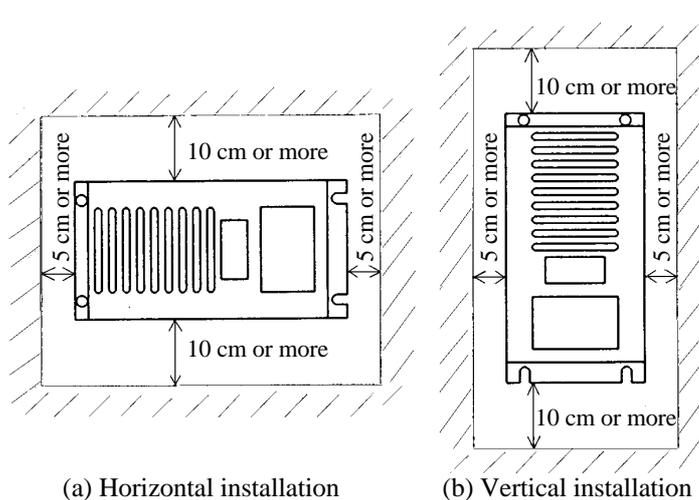
Figure 3.2 Clearance around dynamic braking units EZ2-30K
