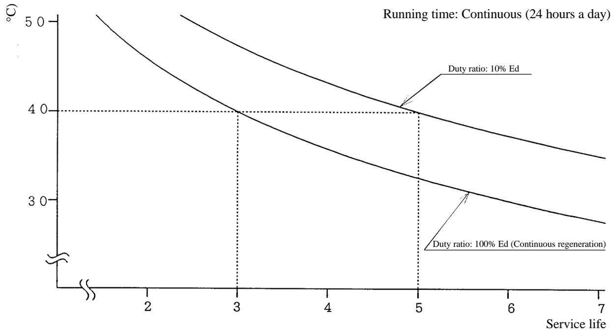
Appendix Figure 1 Ambient Temperature vs. Capacitor Life characteristics
