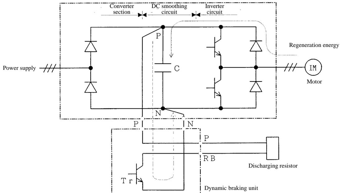
Figure 9.3 Dynamic braking by the inverter
