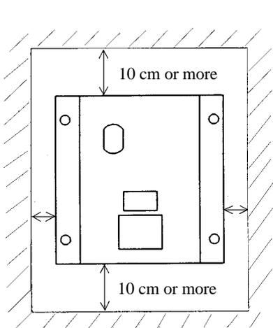
(Never place the dynamic braking unit with its ventilation openings facing left and right.)
