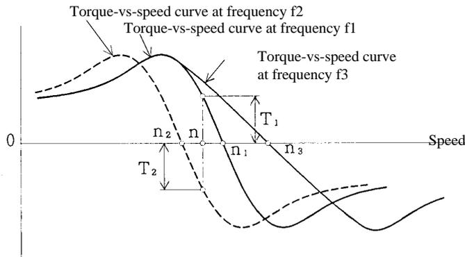
Figure 9.1 Frequency change and motor torque
